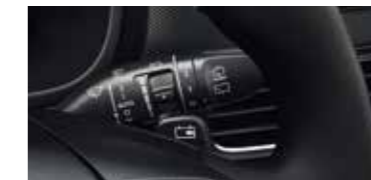
Paddle shifter (Regenerative braking control)
